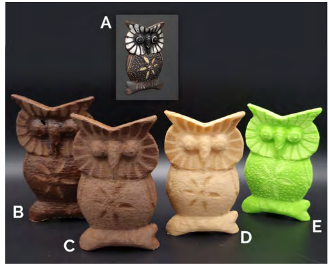
Figure 7: Example of a scanned figurine processed using our method and fabricated with local shade variations. A) The mesh file with texture. B) A print made with Corkfill. C) Another print with Corkfill but with reversed brightness values. D) Print with Woodfill. E) Print with green LW-PLA.
