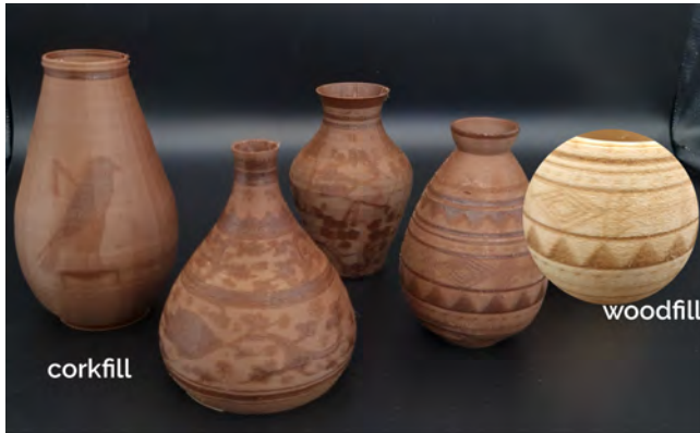
Figure 6: Examples showing local shade variations. Each object was printed using a single material; either Corkfill or Woodfill was used.
