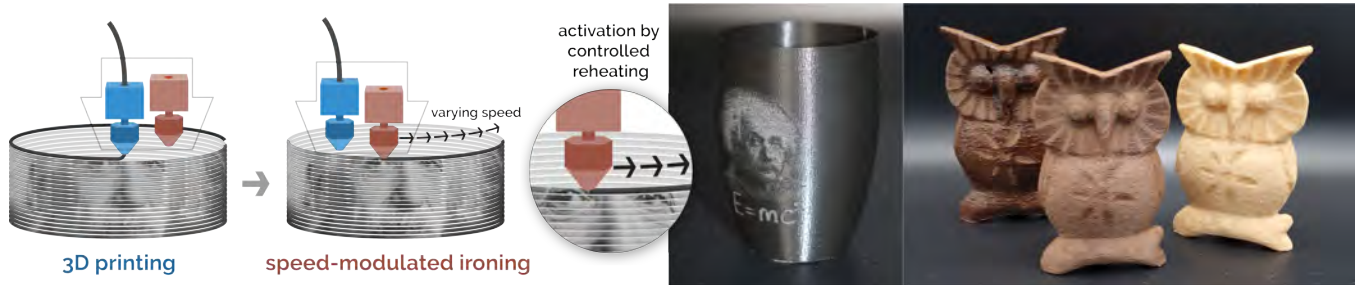
Figure 1: Speed-Modulated Ironing is a novel 3D printing technique for FDM 3D printers to continuously program visual and tactile properties at a high resolution. It works by using one nozzle to lay down the filament, followed by the second nozzle that activates the temperature response of the material by "ironing" the printed layer at varying speeds, changing the achieved property. Our method can be used for different temperature-responsive filaments.
