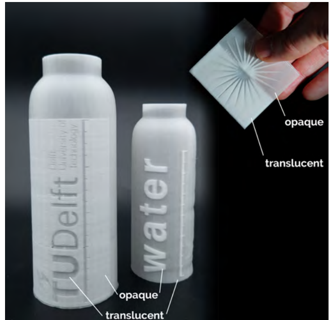
Figure 8: Liquid containers printed using "natural color" LW-PLA. Regions ironed at a low speed become opaque, while regions ironed at a high speed remain translucent.
